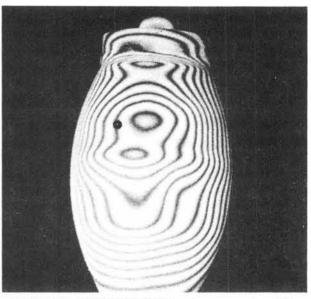
RESIDUAL DEFORMATION of a good-quality vessel. Fringe pattern indicates that maximum expansion occurred near center of vessel.
